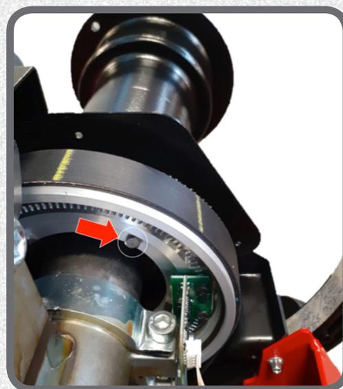
If these screws are black (ferromagnetic burnished steel), they must be replaced with other screws of the same size in non-magnetic STAINLESS steel (VTE M4X10).
