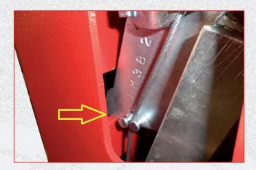
In the lower internal part of the columns, apply a load of approx. 3 kg to the end of the rope to tension it.
