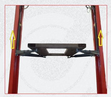
Operate the lever, lower the trolleys until reaching the first upper safety tooth.
