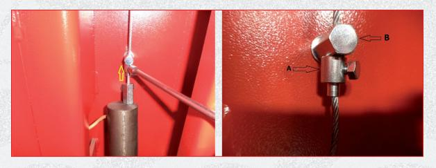
To check that the ropes are properly tensioned, move the trolleys up using the up button on the electrical panel. With trolleys stopped, press and hold the yellow button.
