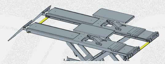
**TECO 4500C, TECO 4500C CT, TECO 4500C CT LT** versions: New models with capacity 4,5 T and platform length 4.200 mm, added to the price list since September 2022
