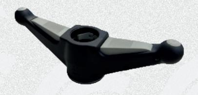
The new nut can be interchanged with the previous version. The central diameter and thread pitch are Ø40 x 3mm.
